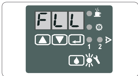
FLL: Fault Low Level (fill level too low)
