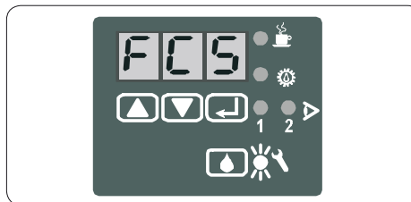
Fault notification on device display
